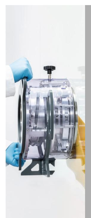
PIERCAN presents and innovative, unique and patented solution: the STIC System allows the change of gloves or drybox accessories in a fast and secure way.
