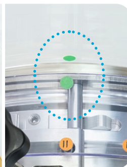
2 • Position the barrel on the BE , respecting the alignment of the marks. The lever is now in position I.
