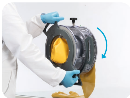
4 • Replace the BS by turning the wheel clockwise with the handles until it stops. The SB and its used accessory are ejected into the glove box. The new BS is immobilized.
