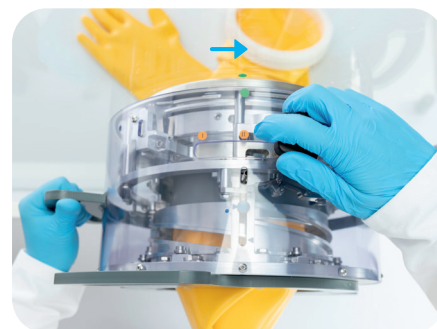
5 • Remove the barrel by moving the lever to the right (position III). Remove the barrel, the change is complete.
