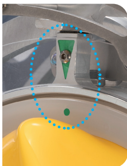
1 • Position the BS in the barrel, respecting the alignment of the marks.
