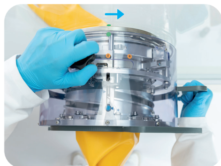
3 • Lock the barrel by moving the lever to the vertical position (position II).
