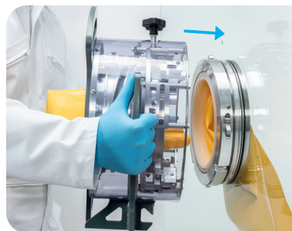
2 • Position the barrel on the BE , respecting the alignment of the marks. The lever is now in position I.
