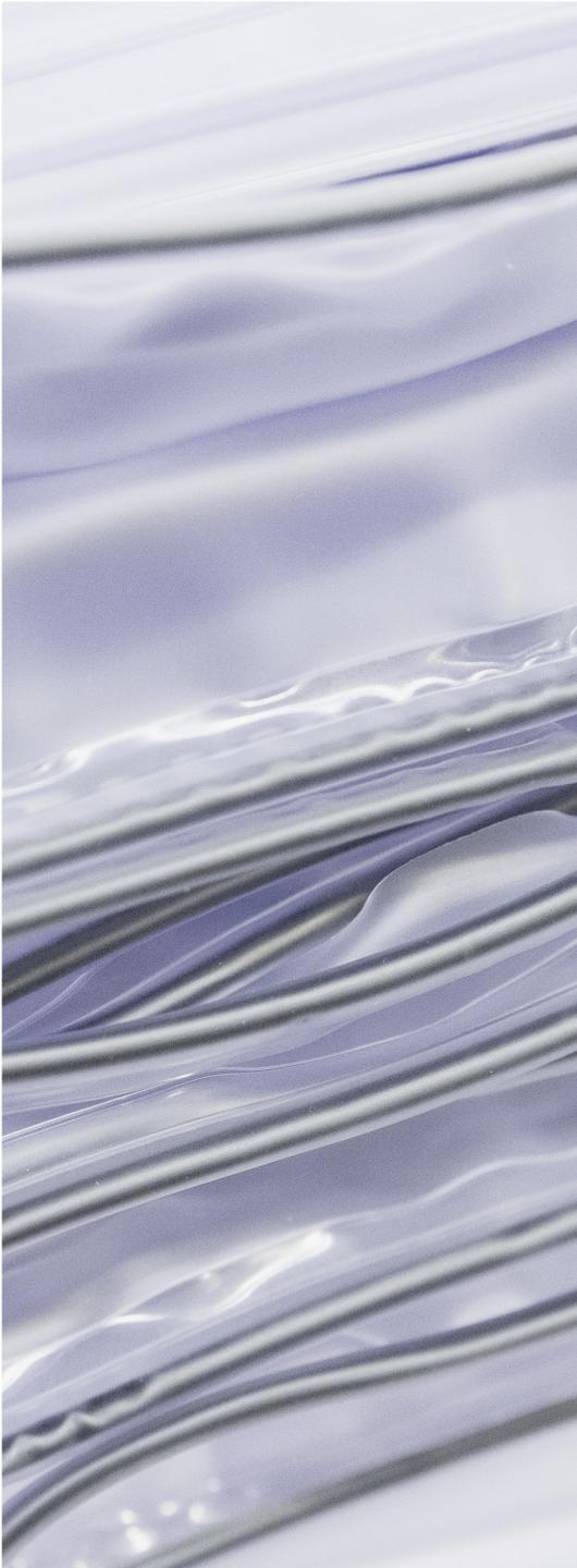
**Flexible polyvinyl chloride film** – PVC, transformed by calendering. **Compatible** with **cleaning agents, decontamination** and **disinfection**. Welds adapted to manipulations in glove boxes and isolators: **resistant, soft, smooth, elastic** and **waterproof**.
