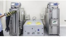
• Glove integrity testing: 100% are checked. Each glove is leak tested under negative pressure in line with the standard EN 421.
