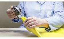
• **Beading check:** By sampling, 1 glove per box. At the mid-point between the sides and at the fold of the glove.
