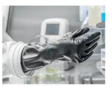
PIERCAN offers a patented and innovative solution, developed by its research and development laboratory: the securised glove port (BCS, bague de connexion sécurisée) that allows changing gloves without loss of containment.
